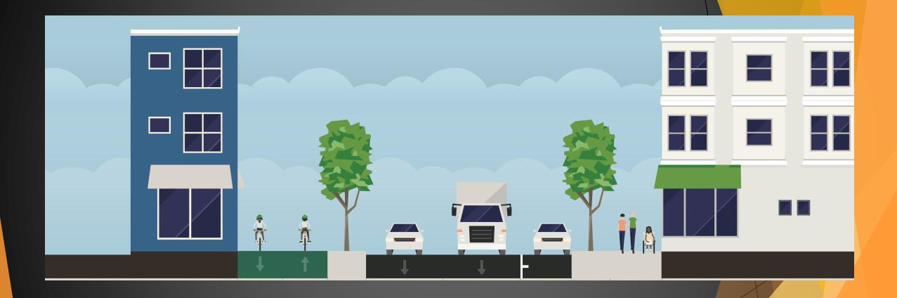
Reconstructs curbs, removes one travel lane, relocates parking.
