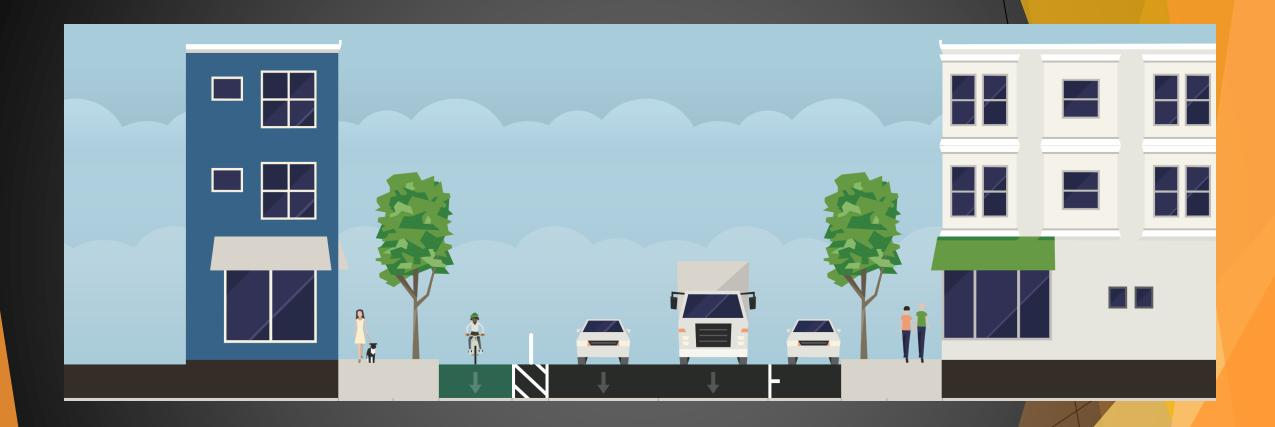
Maintains existing curbs, removes one travel lane, relocates parking.
